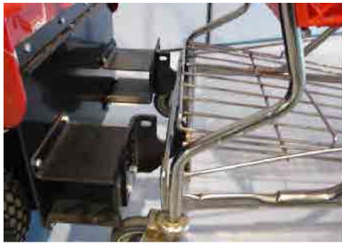
Fig 3. Style 1 Cart. Place rearmost horizontal bar in Yoke grooves.
