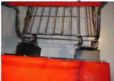
Fig 5. Affix Locking Pins to complete Lead Cart Installation.
