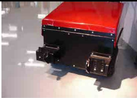
Fig 1. Affix Left (220-094) and Right (220-095) Drop-In Yokes to QuickKART as shown above using 4 Bolts (400-013) provided.
